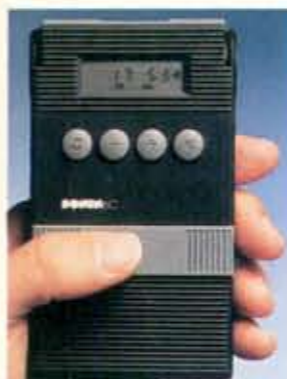
HOW NEAR, HOW FAR Unlike many computerish gadgets, the handsome Sonin is authentically useful. Produced by Sonin Inc. and Pentagram Design/L.D.Works, the sonar device, when pointed at a wall or ceiling, calculates the distance (up to 250 ft.) instantaneously. The swiveling, rolltop-desk-like lid is also an on-off switch.
