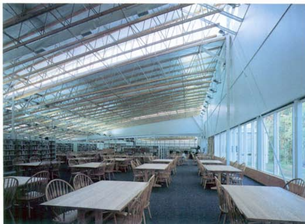
Left, the main reading room in the building's southeast corner. Below left, a trio of windowed study cubicles on the south wall. Right, the periodical area adjacent to the major east-west axis. Bowed warren trusses have wood cords and galvanized steel webs; lights are standard stadium fixtures. □
